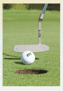
A putter molded by PIM compound which lets the club blade and hozel be manufactured as one piece. Normally the face and hozel pieces are cast separately and brazed together.
