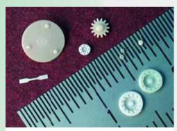
Examples of microcomponents made of zirconium oxide, smallest total diameters are in the range of about 670 µm.
