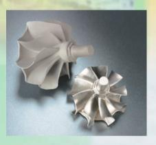
The parts complex 3D shape cannot be reproduced by machining and with fewer production steps, MIM is a viable alternative to investment casting for this high-volume part.
